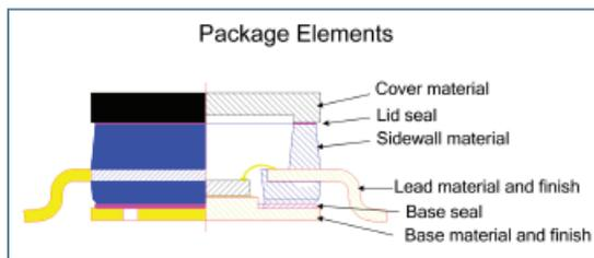
**Figure 1:** ACP packages use an insert-injection molding process that combines a metal alloy lead frame with an LCP sidewall and matching lid with a pre-applied B-staged epoxy.
