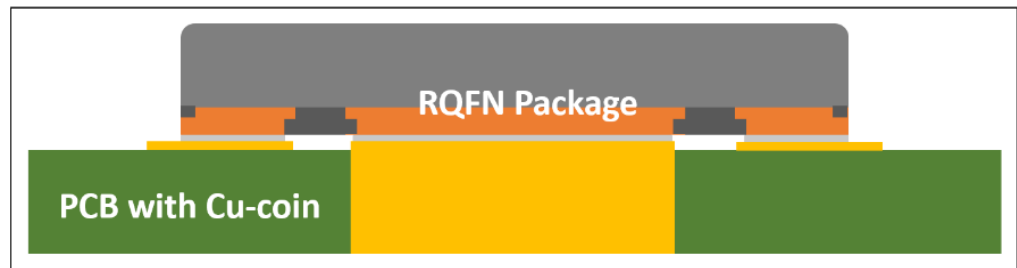
Figure 17: PCB with Cu-coin
