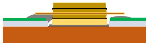
Figure 11: Flange Cavity is Too Shallow
