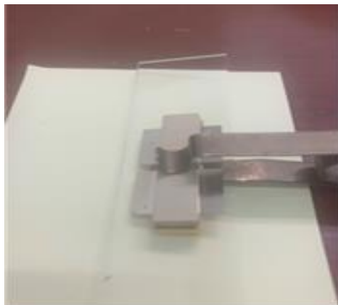
Figure 6. Flange and Ringframe Assembly Clipped with Lids Before Loading to pre-cure and Post cure Oven
