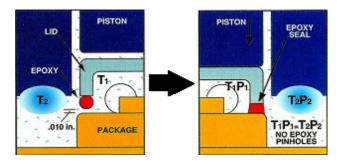
Figure 4. The ITS sealing cycle advantage
