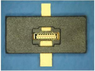
Figure 6. Partially matched microwave package.
