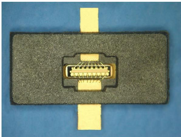
**Figure 6. Partially matched microwave package.**
