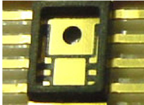
**Figure 7. Sensor package in an SOIC 8 lead format.**
