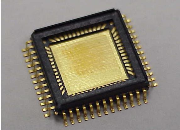
**Figure 8. Quad flatpack optical package with a transparent glass cover**
