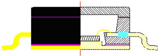
**Figure 2. Representative R-Pak package cross section illustrating the internal cavity with a wirebonded die on a metal package base**
