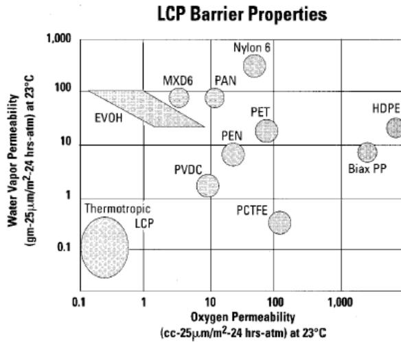
**Figure 3. Water vapor and oxygen permeability of plastics [5]**
