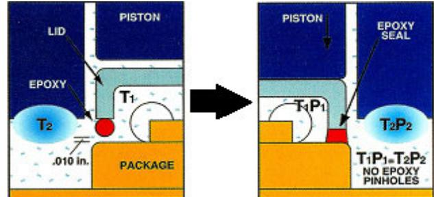
**Figure 4. The ITS sealing cycle advantage**
